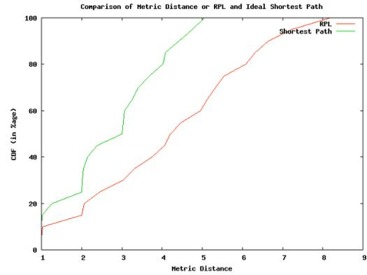
(b) CDF: Total number of ETX to deliver a packet with respect to total path ETX.
