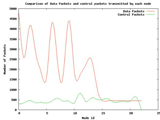
Figure 3: Amount of data and control packets transmitted for each node when minimizing ETX is used OCP along the DAG.
