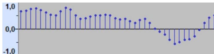
For instance, the first point is 0.68 at time 0. The next point is 0.69 at time 10 milliseconds. The next one is 0.73 at time 20 milliseconds. The time step between points is called the sampling rate.
