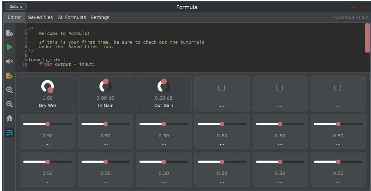
If you are using an existing formula, the formula author should have labelled the knobs and switches his formula is using. Typically, the knobs and switches that have the ... label are not used within the formula.
