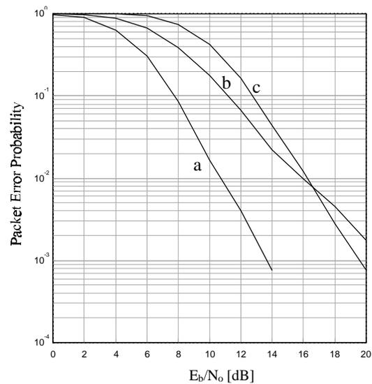
Figure 17: Packet error ratio for a) rate  $1/2$  coding with QPSK, b) rate  $3/4$  coding with QPSK and c) rate  $1/2$  coding with 16-QAM. Packet size is 1024 bits.
