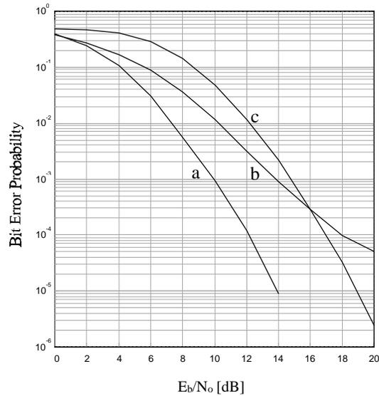
Figure 16: Bit error ratio for a) rate  $1/2$  coding with QPSK, b) rate  $3/4$  coding with QPSK and c) rate  $1/2$  coding with 16-QAM. Results are obtained by simulating 4000 independent Rayleigh fading channels with an exponentially decaying power delay profile. Delay spread is 100 ns.
