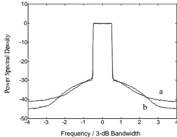
Figure 12: a) plain OFDM with 7.4 dB backoff, b) peak windowing with 5 dB backoff
