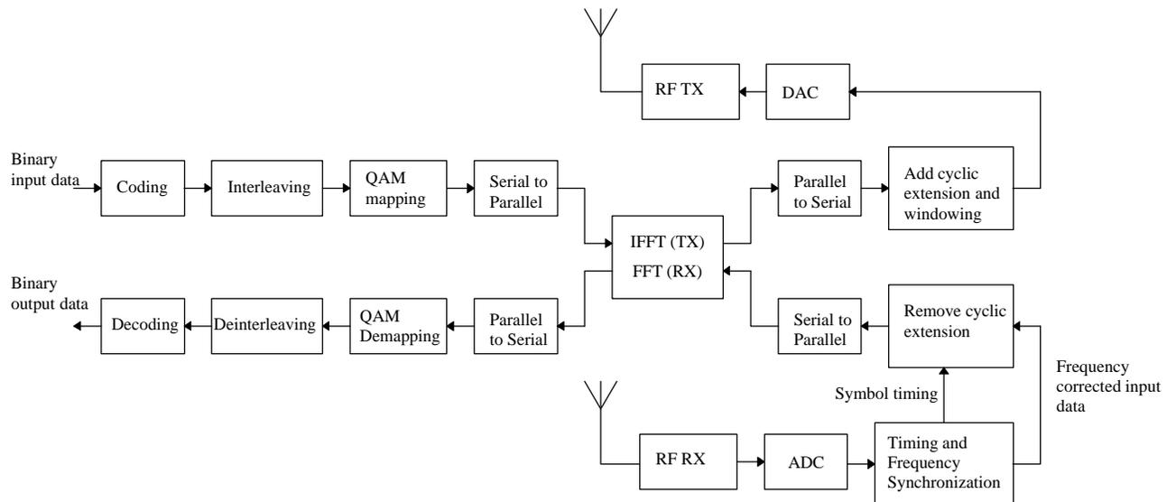
Figure 1: Block diagram of an OFDM transceiver.
