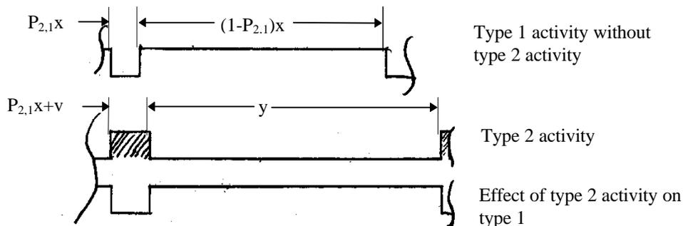
The lower illustration shows the average cycle time when a type 2 system is introduced with a demand which exceeds the capacity available. In this case, when the type 1 traffic becomes inactive, the type 2 system obtains access and uses the capacity for all of the time it would perceive the type 1 traffic to be inactive plus a carry over time of  $v$  seconds which represents the average time the type 2 system continues to maintain access after the type 1 system begins to compete.
