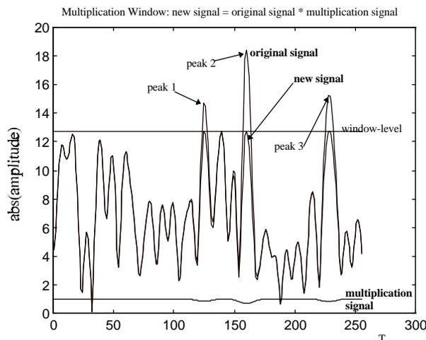
Figure 9: Windowing an OFDM time signal
