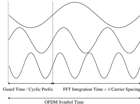
Figure 3 : OFDM symbol structure showing 3 specific subcarriers.
