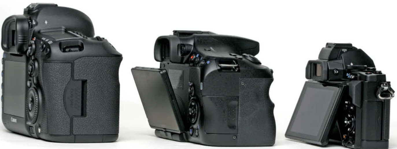
Differing degrees of monitor freedom. From left to right: the Canon EOS 5D Mark III with its fixed monitor, the Sony SLT-A57's tilt/rotatable model and the up/down tilt of the Olympus OM-D E-M5.
