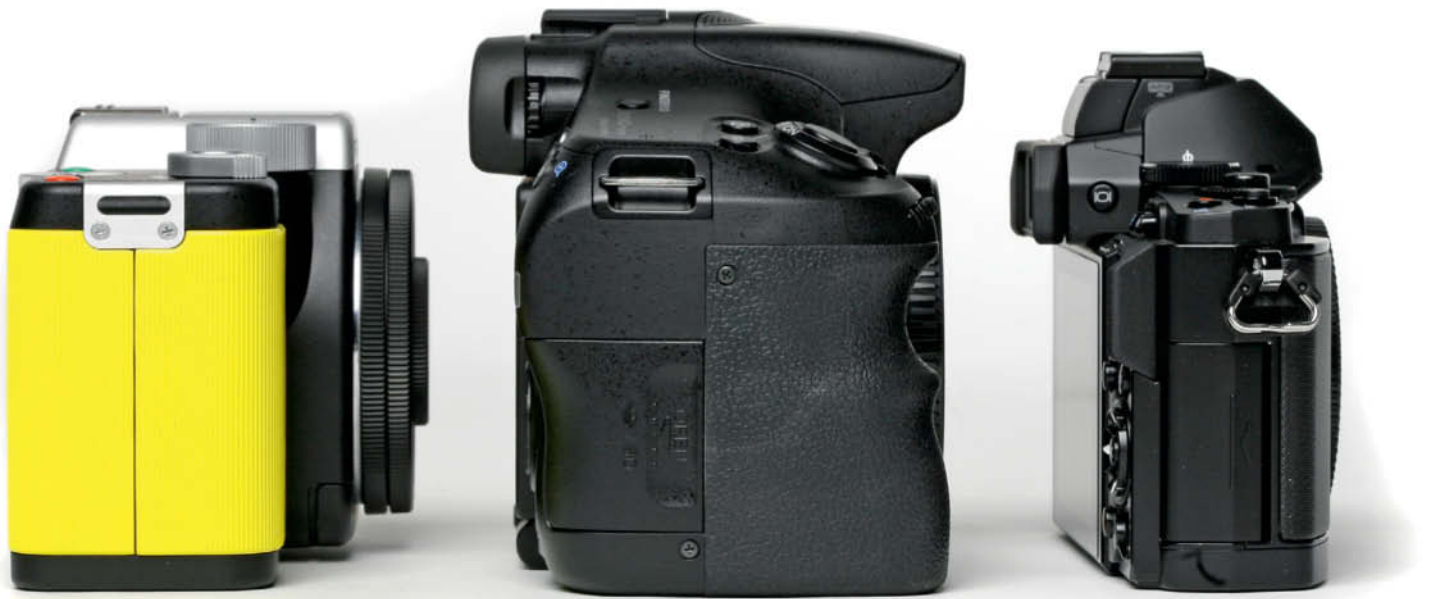
The Pentax K-01 is hardly any slimmer than an APS-C SLR, even though it has no mirror. On the plus side, it is compatible with all Pentax K-mount lenses. The Olympus OM-D E-M5 with its much smaller Micro Four Thirds body is shown on the right.
