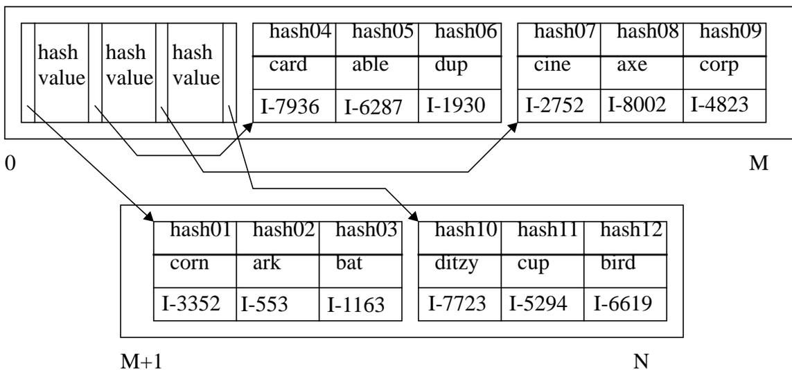
The B-tree is embedded inside a linear array of blocks, ie: a file structure. Pointers to B-tree blocks are relative to the file, not to the filesystem.
