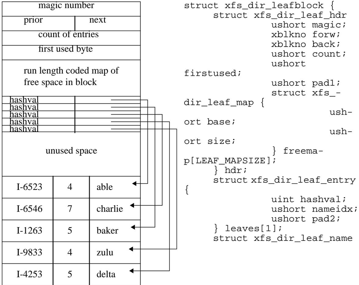
Packed at the front are the hash value and offsets of each of the strings. The entries are sorted on hash value. Packed at the back are the inode numbers, string lengths, and the strings themselves.
