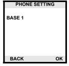
7 Use the numbers on the V-250's keypad to enter the base station PIN. This is a 4 digit number you configure on the base station. Press the **Right Softkey** to select **OK** and enter the screen to enter the base station PIN (password). Default on ZyXEL base stations is **1234**.
