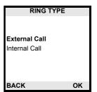
3 Use the Navigator-up and Navigator-down keys to select internal or external call settings. Press the Right Softkey to select OK with one of the types of calls selected (for example External Call). The LCD displays as shown.
