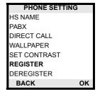
6 Use the Navigator-up and Navigator-down buttons to scroll and select which base station you want to register with (1-4). You can register with up to 4 base stations. Press the Right Softkey to select OK and enter the screen to enter the base station PIN (password).
