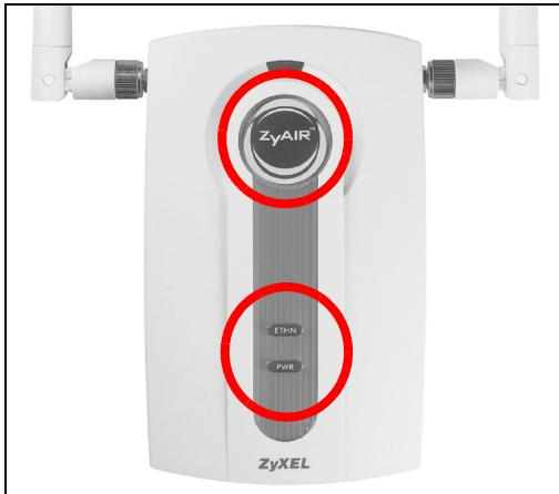
The **PWR** and **ZyAIR** LEDs turn on when the power is connected. The **ETHN** LED turns on if the **ETHERNET** port is properly connected.
