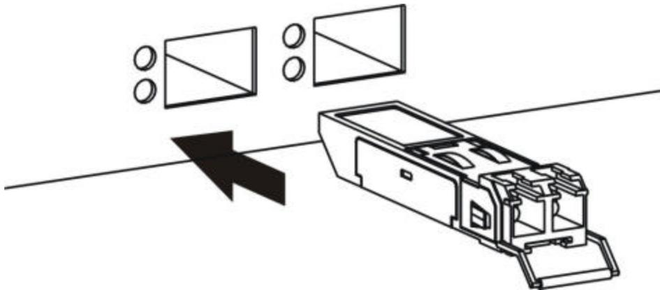
**Figure 3-2 Transceiver Installation Example**
