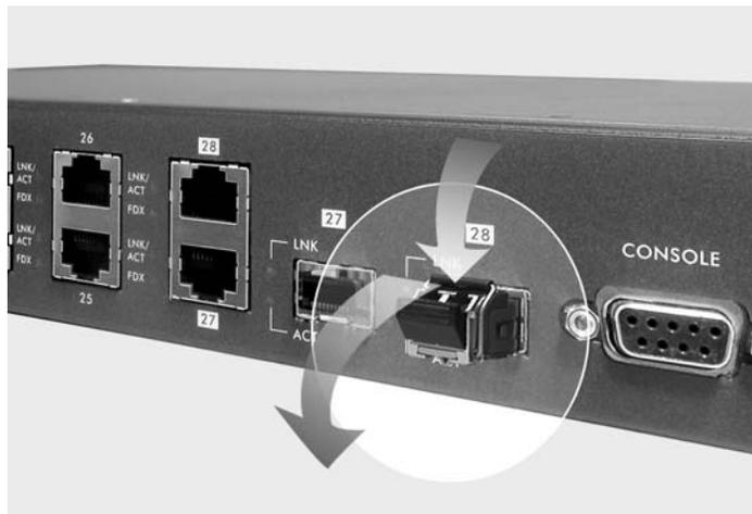
**Figure 3-4 Opening the Transceiver's Latch Example**
