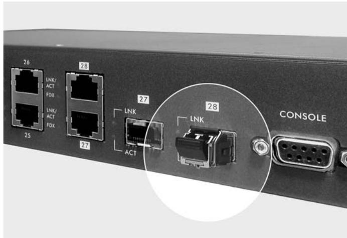
**Figure 3-3 Installed Transceiver**
