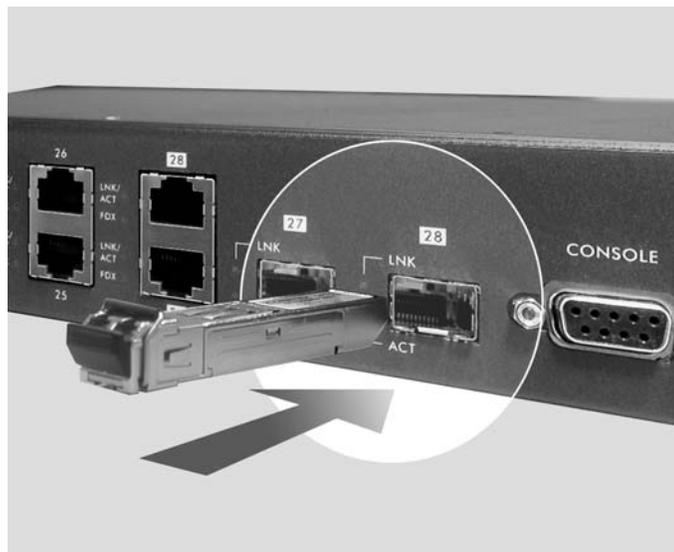
**Figure 3-2 Transceiver Installation Example**
