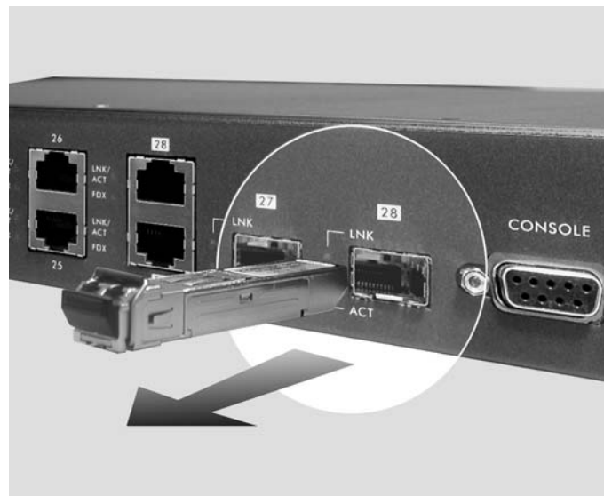
Figure 3-5 Transceiver Removal Example
