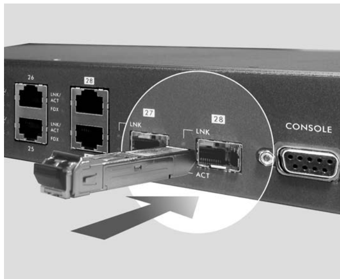
Figure 3-2 Transceiver Installation Example
