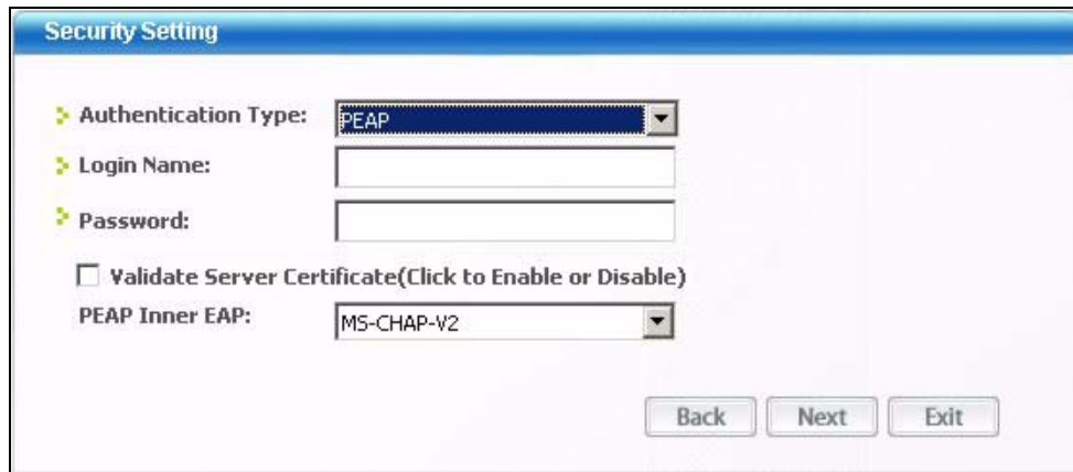
Figure 29 Station Mode: Security Setting: 802.1x
