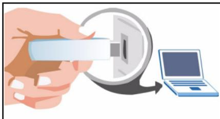
Never bend, twist or force the AG-225H v2 into the port. If there is not enough space to attach the AG-225H v2, use the included USB cable.
