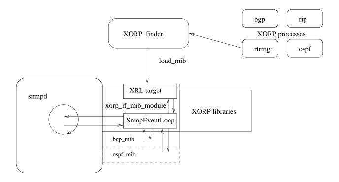
Figure 1: Functionality of xorp\_if\_mib\_module
