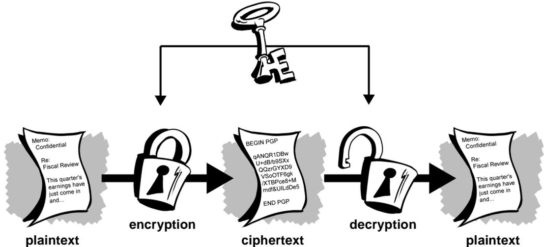
Figure 1-2. Conventional encryption
