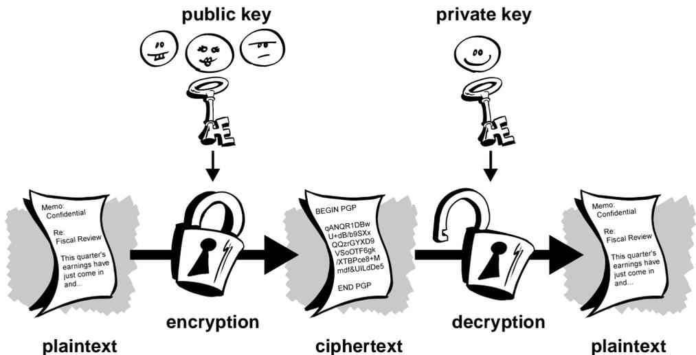
Figure 2-1. Public Key Cryptography diagram
